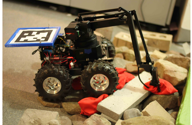
Fig. 1: Low-cost mobile manipulator made from off-the-shelf components that can handle (pickup/drop) compliant bags and navigate over unstructured terrain.
