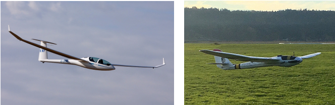
Fig. 2: A full-size DG1000 sailplane (left, photo credit: Paul Hailday ) and Radian Pro remote-controllable model sailplane that serves as our sUAV platform (right).
