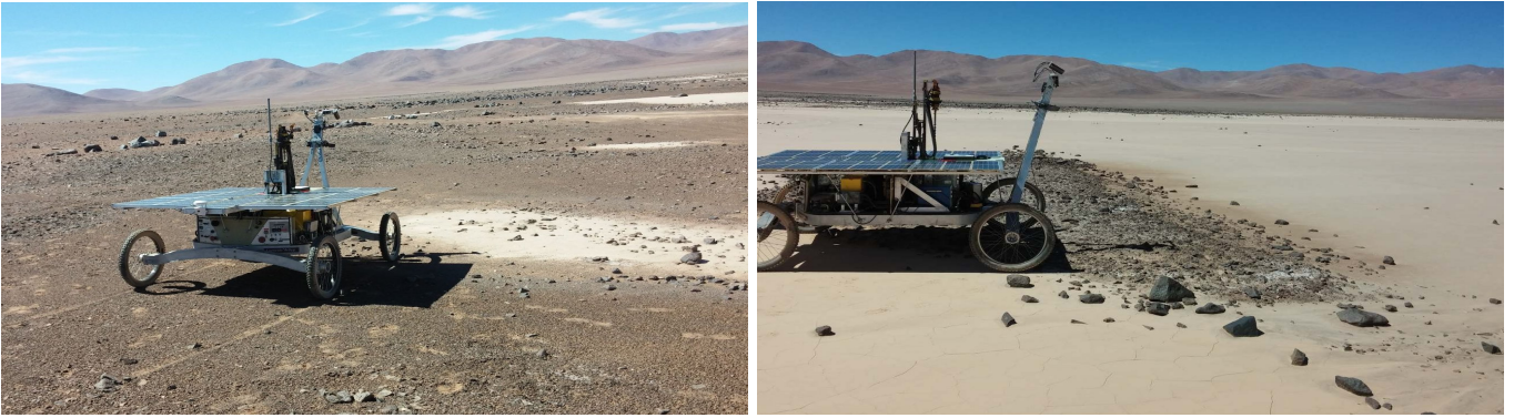
Fig. 1. Two instances of where better target selection could have improved robotic sample selection. In both situations the robot navigates to a location and collects a grid of spectra immediately in front of it. In the left image it has correctly identified a region of interest and navigated there, but is pointing in an incorrect direction and samples from a mixture of the materials. In the right image it has again navigated to the correct location but aims its spectrometer beyond the optimal targets, including patches of white salts that are of interest to the science team.
