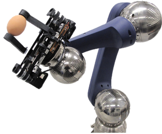
Fig. 1. The variable stiffness gripper with antagonistic magnetic springs.
