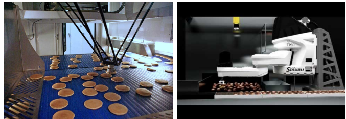
Fig. 1. Examples of robots deployed in industrial settings tasked to arrange objects in desired configurations through pick and place: (left) ABB’s IRB 360 FlexPicker rearranging pancakes (right) Stäubli’s TP80 Fast Picker robot.
