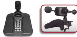
Fig. 5. A 2-axis joystick (left) and switch-based head array (center) and their operational paradigms (right). v and \omega indicate the translational and rotational velocities of the end-effector, respectively.
