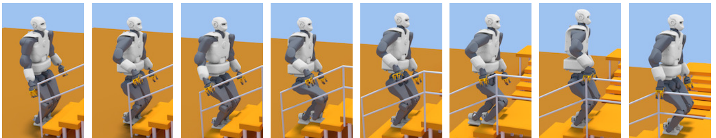
Fig. 8. Snapshots of the climbing 15-cm high steps motion with guardrail by the TALOS robot in simulation.
