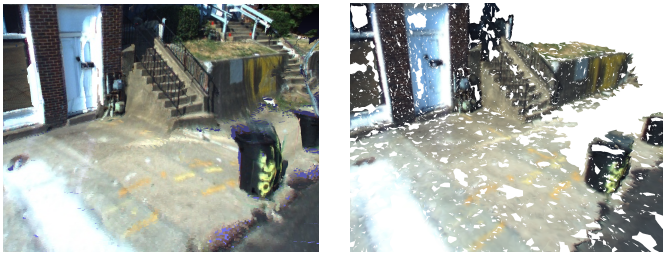
Fig. 7. Qualitative comparison of dense 3D reconstruction. Left: Our method. Right: PMVS results after ball pivoting surface reconstruction. Our approach is denser and one order of magnitude faster to compute (26 \times ).
