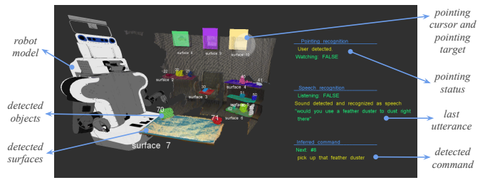
Fig. 4: LUCIT’s visualization which provides additional transparency about its internal processes including speech recognition, pointing detection, scene understanding, and command inference.
