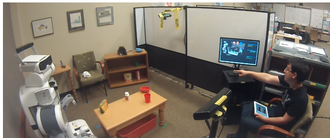
Fig. 1: LUCIT combines speech recognition , pointing detection , and scene understanding to interpret situated natural language commands. LUCIT’s transparency mechanisms allow the user view to the output of these intermediate internal processes.
