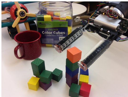
Fig. 1. A Baxter parallel gripper enhanced by two arrays of combined force and proximity sensors. Seven sensors are spaced along each finger’s contact area, and one sensor is mounted at each tip, enabling object detection and force control.
