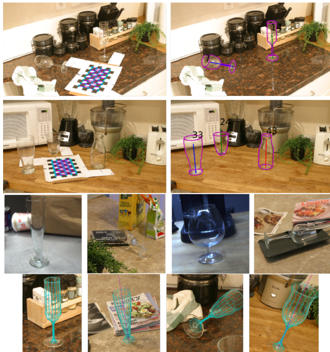
Fig. 1: Annotated multi-view transparent dataset. The first two rows each show a single viewpoint, with and without the calibration pattern used to annotate groundtruth camera and object pose. Example outputs The last row shows models and poses automatically recovered by the proposed approach.
