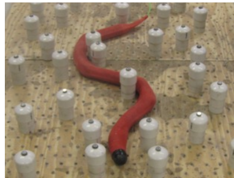
Fig. 1: Snake-like robot autonomously moving through a peg array with no a priori knowledge of the array parameters.
