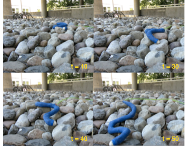
Fig. 7: Autonomous locomotion over unknown rock pile using torsional shape compliance. A video of this behavior appears in the supplemental material.
