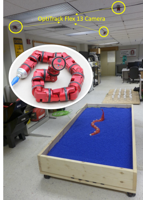
Fig. 1. A snake robot on a bed of small plastic spheres. The cameras mounted to the ceiling track the robot’s position changes as it changes shape. The joints on the snake are series-elastic actuators that allow for force measurements.
