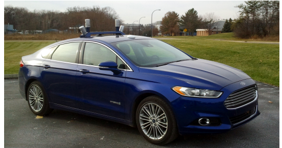
Fig. 3. Our autonomous car platform, used to record the traffic-tracking dataset we use in this work. The vehicle is equipped with a sensor suite including four LIDAR units and survey-grade INS.
