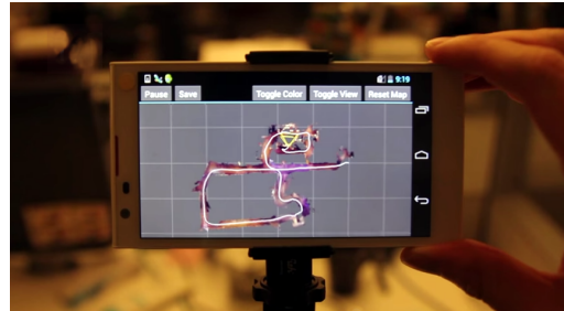
(a) CHISEL creating a map of an entire office building floor on a mobile device in real-time.
