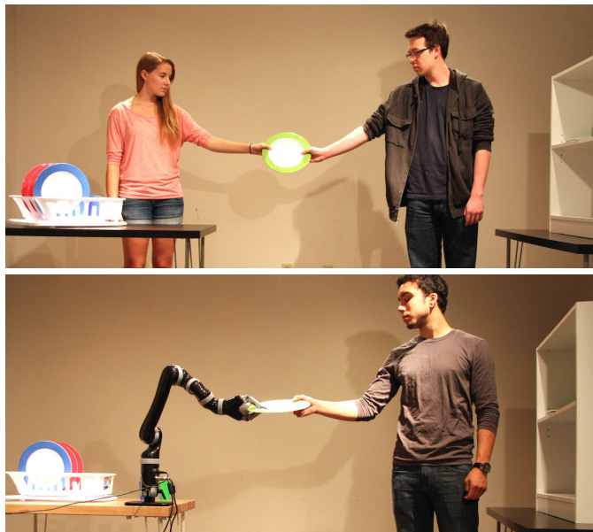
Fig. 1: We studied human-human handovers (top) in a household scenario, identified strategies that humans used for coordination, implemented them on an robotic manipulator, and evaluated their effectiveness in supporting coordination in human-robot handovers (bottom).
