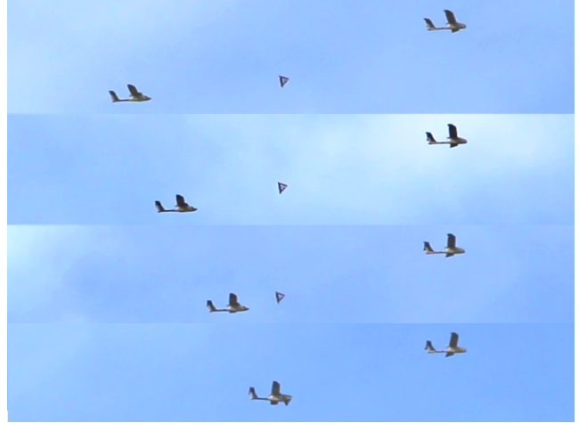
Fig. 1: The terminal approach to docking with a towed drogue.
