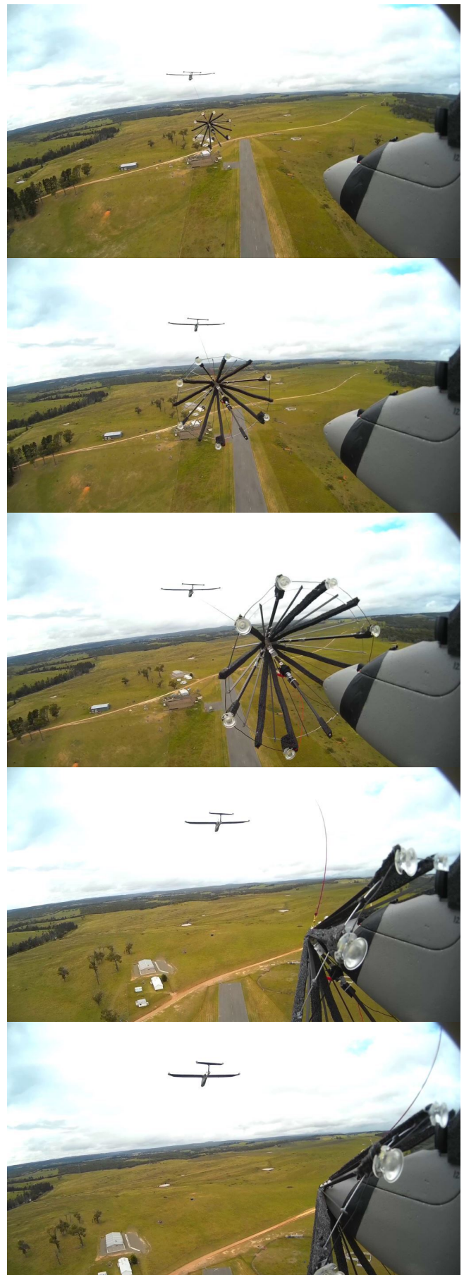
Fig. 10: The approach to docking, then station keeping, taken from the left wing of the follower.
