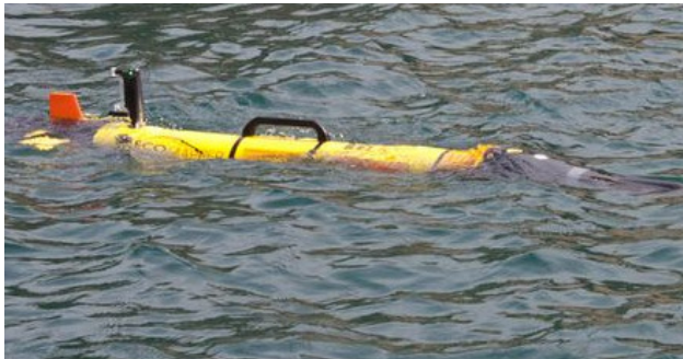
Fig. 4. Ecomapper propeller-driven AUV used as a surface vehicle for lake monitoring experiments with the proposed ReASC adaptive classification algorithm.
