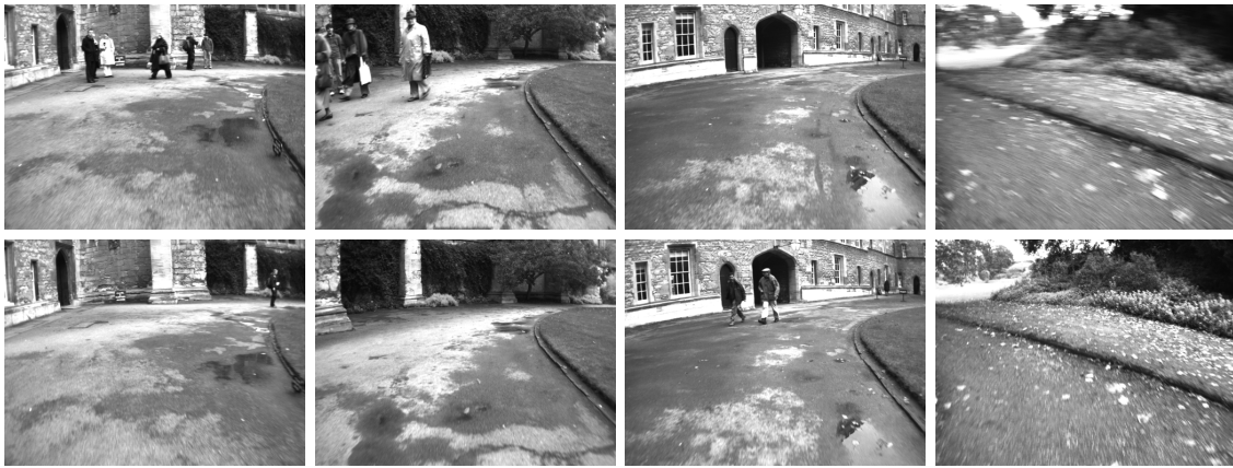
Fig. 1: Sample images from the New College dataset: Query images (top) and the corresponding match images(bottom). The images are down-sampled to 8 \times 6 pixels. Note that in spite of dynamic changes and motion blurs occurring in these images which deteriorate the loop-closure problem, the proposed approach still provides reliable results.
