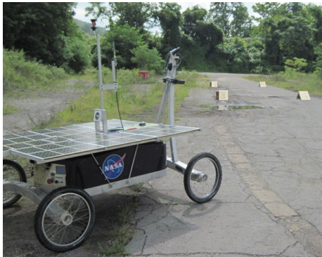
Fig. 4. Photograph of the test rover and four ramp obstacles at the Robot City test location.
