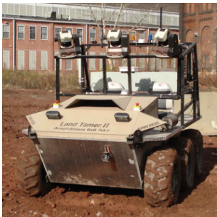
Fig. 6. The LandTamer (made by PFM Manufacturing Inc.) is a six-wheeled skidsteer platform.
