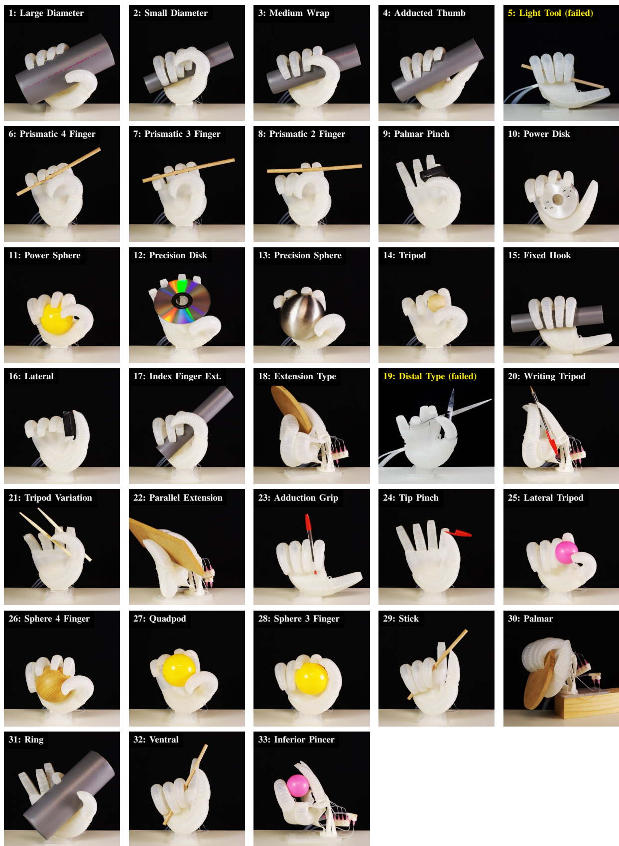
Fig. 10. Enacted grasps of the Feix taxonomy, using empirically determined actuation patterns: Grasps are numbered according to the Feix taxonomy [11]; the hand failed to replicate grasps 5 (Light Tool) and 19 (Distal Type, Scissors)
