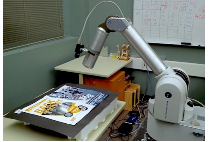
Figure 6. Experimental setup for a visual servoing experiment using the WAM arm with a wrist-mounted camera. Patches of a highly textured surface in the camera’s field of view were tracked and used as input to a visual servoing routine in order to precisely align the camera position. The algorithms were compared based on the speed and reliability of the overall system.
