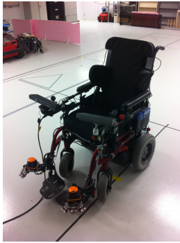
Fig. 4. Picture of the robotic wheelchair equipped with Kinect
