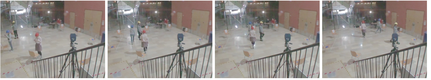
Fig. 2. Recording real-world training data: The figures show snapshots of three human subjects avoiding each other in order to proceed to their next target location. Using a motion capture system, we recorded one hour of human interactions by tracking markers that were attached to hats worn by the subjects. To prevent the subjects from focussing on their walking behavior, which may result in awkward trajectories, we made them read and memorize newspaper articles at various locations saying that we were conducting psychological research on the effects on attention when frequently changing locations.
