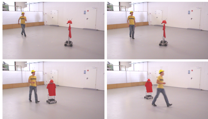
Fig. 1. Encounter of a robot and a pedestrian. A robot that is able to predict the behavior of the pedestrian can navigate in a socially more compliant way.
