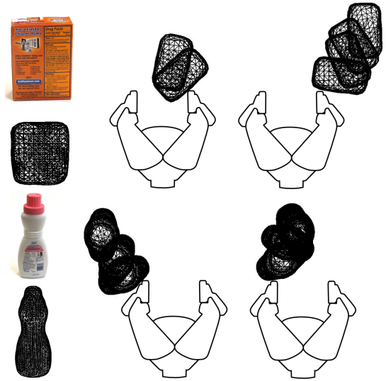
Fig. 2. Left: Example objects and their trimesh models. Right: Examples of computed trajectories of objects as the hand pushes them. The hand motion is towards the top of the page in each diagram, and is not shown.
