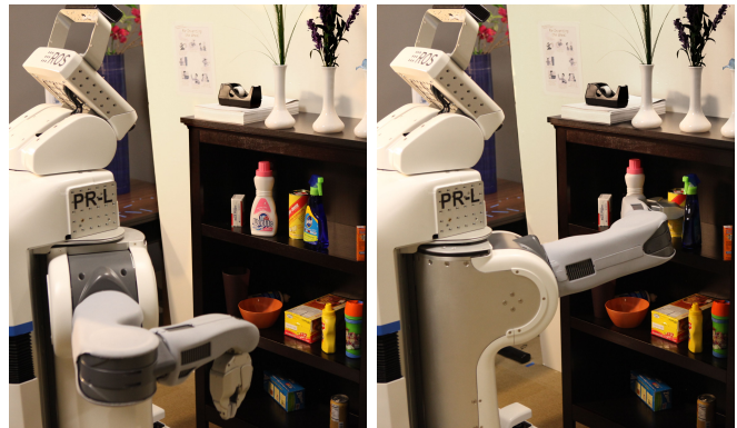
Fig. 1. Manipulation in a constrained and cluttered environment. Left: a robot tries to acquire a partly occluded object from a constrained shelf space. Right: the robot clears a path to the target by pushing obstacles in a controlled manner, and completes the grasp.
