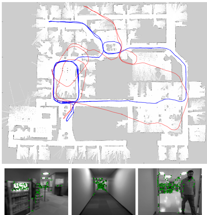
Fig. 1. Top: Skeleton map constructed online from just stereo images, registered against a laser map for reference. Red is visual odometry, blue is corrected by loop closure from visual place recognition. Tick marks at sides of map are 10m intervals. Bottom shows typical views, with blurring, clutter, people, and blank walls.
