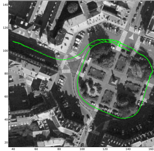
Fig. 7. Versailles Rond sequence of 700 video frames taken from a moving vehicle, 1m baseline, narrow FOV. (Dataset courtesy of Andrew Comport [7]) Top: matched loop closure frames. Bottom: top-down view of trajectory superimposed on satellite image.
