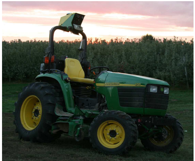
1: A John Deere tractor (4710 series) was used for some of the experiments in agricultural applications. It was equipped with cameras, positioning sensors, a computer and a SICK laser for perception.
