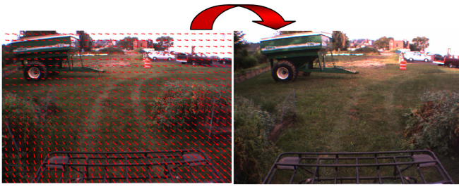
8: Left: Flow for every 16 \times 16 pixels patch to match patches in the right image. Right: Reference image.
