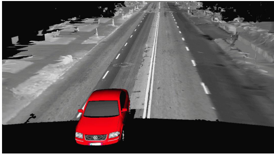
Figure 2. Visualization of the scanning process: the LIDAR scanner acquires range data and infrared ground reflectivity. The resulting maps therefore are 3-D infrared images of the ground reflectivity. Notice that lane markings have much higher reflectivity than pavement.
