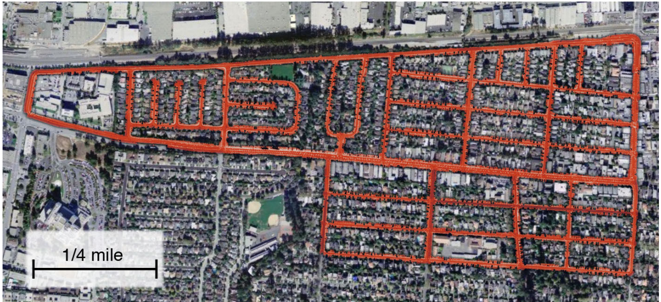
Figure 5. (Best viewed in color) Aerial view of Burlingame, CA. Regions of overlap have been adjusted according to the methods described in this paper. Maps of this size tend not to fit into main memory, but are swapped in from disk automatically during driving.
