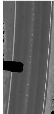
Figure 9. Filtering dynamic objects from the map leaves holes (left). These holes are often filled if a second pass is made over the road, but ghost images remain (center). After SLAM, the hole is filled and the ghost image is removed.
