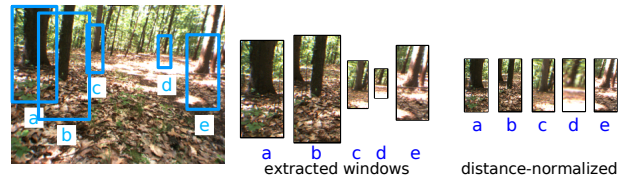
Fig. 3. This figure demonstrates the problem of distance scaling. left : The trees in the image vary widely in size because of different distances from the camera. This makes near-to-far learning extremely difficult. center and right : If windows are cropped from the image and resized such that the subsampling is proportional to their distance from the camera, then a classifier can train on more uniformly sized and positioned objects.
