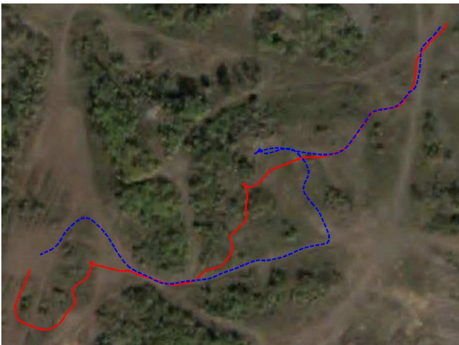
Fig. 6. Comparison of paths executed by our unmanned ground vehicle for shown course when using only on-board perception (in solid red) and with our online learning algorithm used in real-time on-board the robot (in dashed blue). Notice how the online learning path quickly learns to avoid the difficult area near the cul-de-sac and instead chooses to follow the road to the goal.
